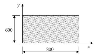
A rectangular, flat plate 800 mm x 600 mm is built up from 8 unidirectional plies of fibre reinforced composite material. Each ply has thickness h = 1.0 mm and the following elastic properties:
