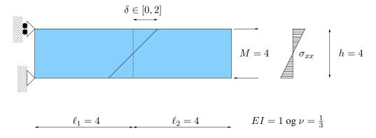
Analyze the problem using two PLANE42 og PLANE82 elements. Vary the  $\delta$  between 0 og 2, i.e. move two nodes. Compare the answers to the exact stress variation.
