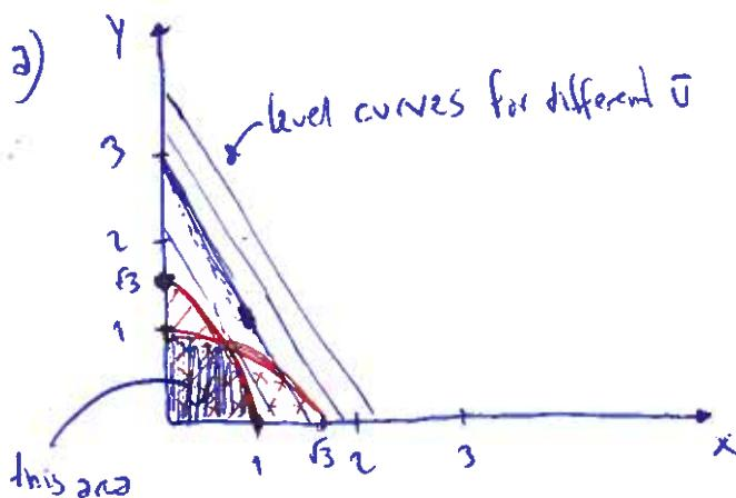
Draw the constraint curves by checking ~~the~~ extreme cases  $x=0$ , and  $y=0$ , then draw smooth curve between (the constraints are of a so called elliptic form, that is the equations are elliptic).
